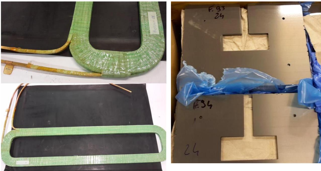
*Fig. 3 Components of the new pulsed dipole for the splitting the BTF beam-lines.*
