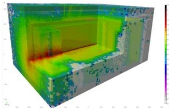
Fig. 2 New BTF bunker simulated dose rate with FLUKA.
